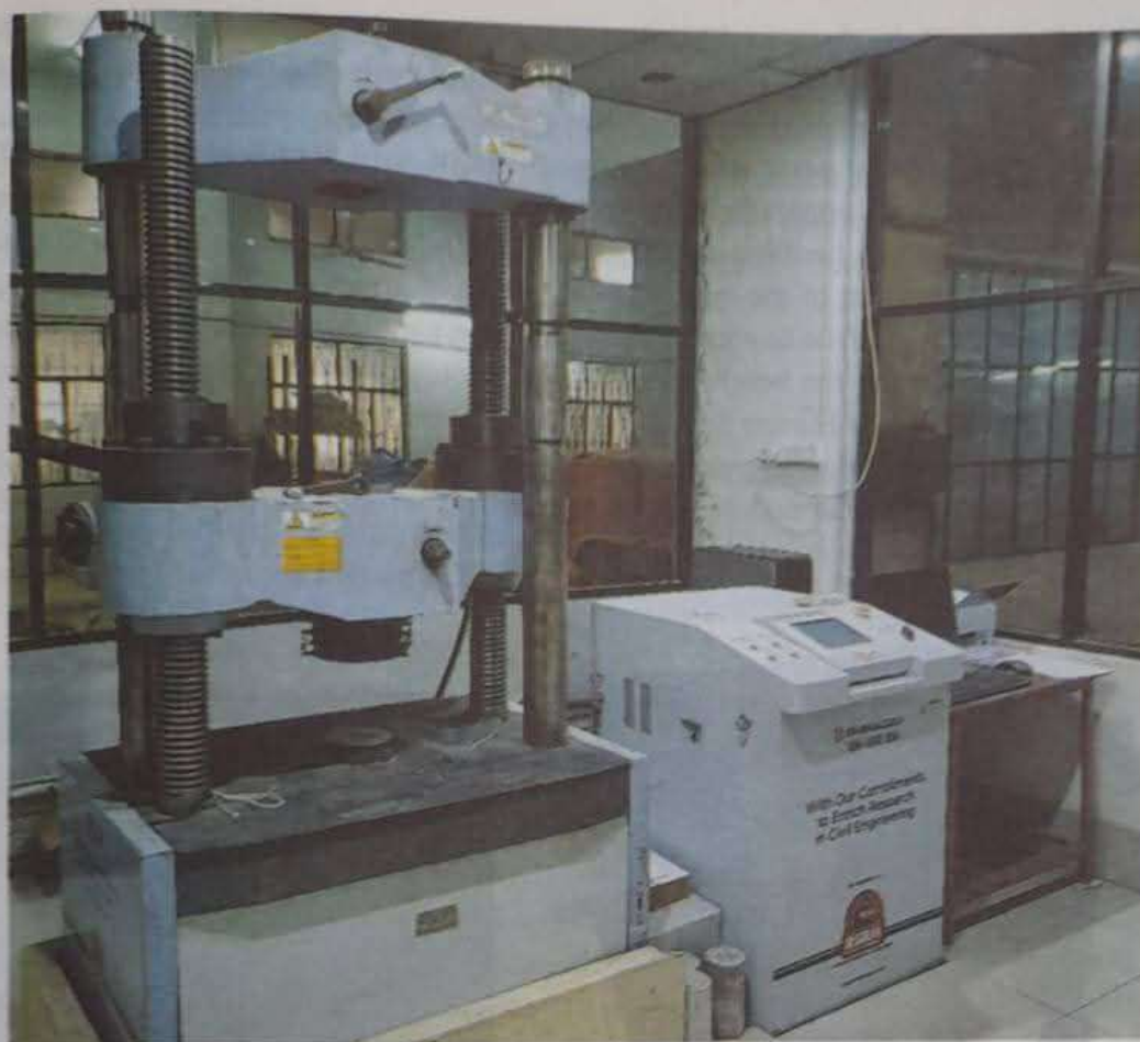
FIGURE 3.3 A modern 100-ton capacity universal testing machine.
